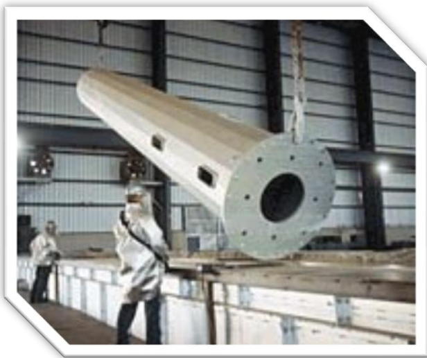
Figures above show the process of dipping steel sections in the zinc bath to galvanise.
