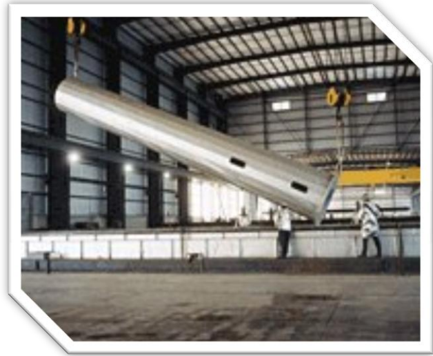
Figures above show the process of dipping steel sections in the zinc bath to galvanise.
