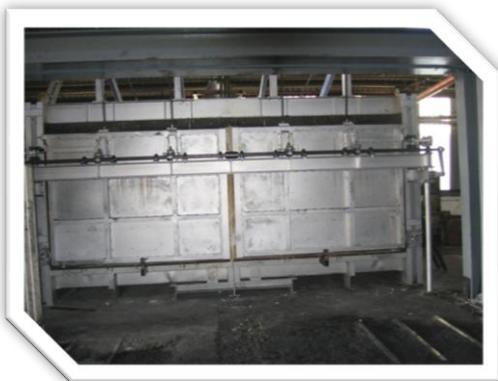
Fig.1 Split door reheating furnace
