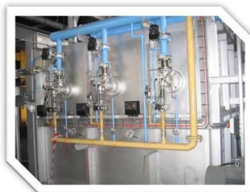
Fig. 2 Burners on reheating furnace
