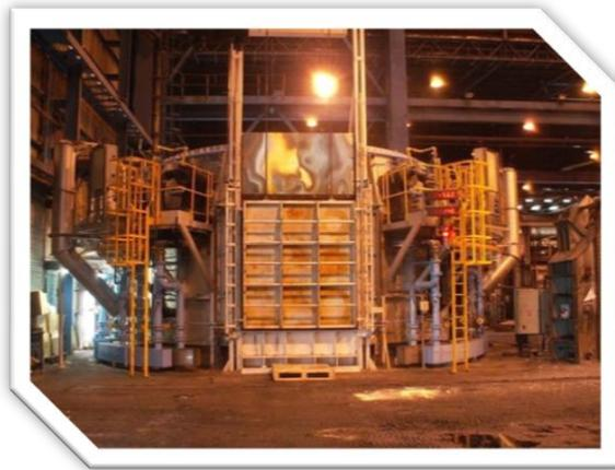
Fig.2 Rotary hearth furnace with the door closed
