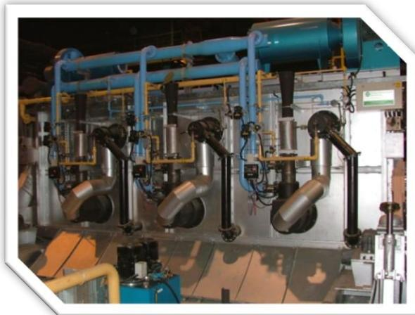
Fig.3 Furnace burners & recuperators
