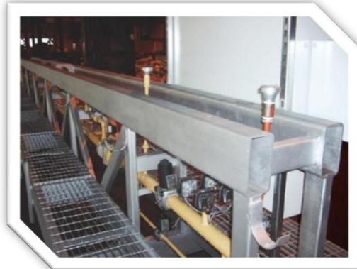
Fig.2 Preheat rig showing gas controls
