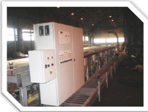
Fig.1 Preheat rig showing control panel
